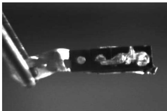
Fig. 14. A photograph showing two tear samples stuck together by melted aluminium.
